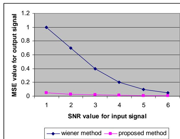
**Figure 5.** MSE values in Wiener method in comparison to proposed method in a Multi-component signal de-noising.
