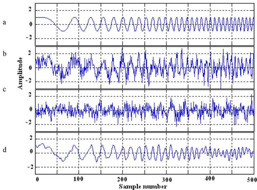
**Figure2.** Comparison of Wiener filter and the proposed method for a FM signal in noise reduction. a)original signal b)noisy signal with Gaussian noise(SNR=1) c) result of the wiener filter d)result of the proposed method.
