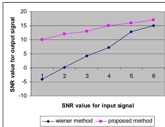
**Figure 4.** SNR values in Wiener method in comparison to proposed method in a FM signal de-noising.
