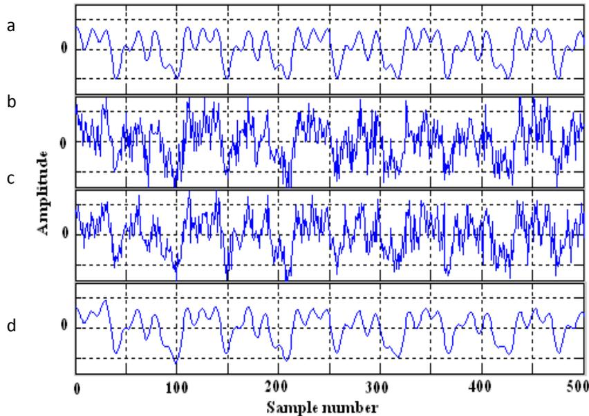
**Figure1.** Comparison of Wiener filter and the proposed method on a multi-component signal in noise reduction a)original signal b)noisy signal with Gaussian noise(SNR=1) c) result of the wiener filter d)result of the proposed method.
