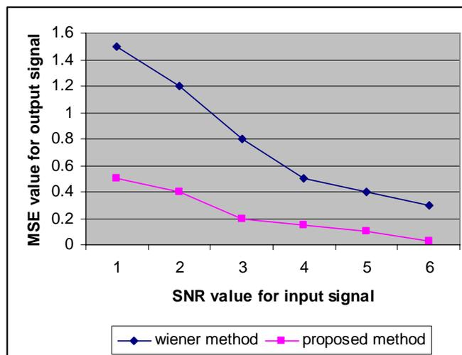
**Figure 6.** MSE variations in Wiener method in comparison to proposed method in a FM signal de-noising.
