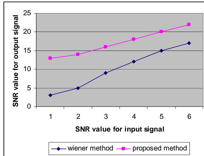
**Figure 3.** SNR values in Wiener method in comparison to proposed method in a multi-component signal de-noising.
