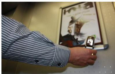
Figure 5: Illustrates NFC's reader mode allows phone to read passive RFID tags on posters. A picture courtesy of NFC Forum
